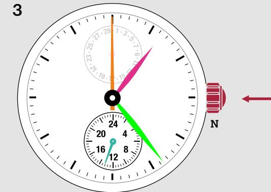
3. Push the crown back to the normal position in accordance with a time signal.
