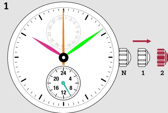
1. Pull out the crown to the second click when the second hand is at the 12 o'clock position.
