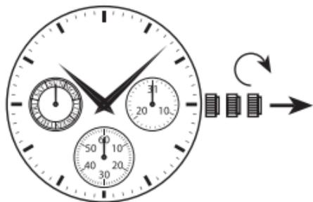
1. Pull out the crown to the second click when the small second hand is at the 12 o'clock position.
