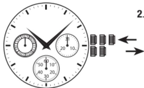
2. Push the crown back in to the normal position in signal. Pull out the crown to the first click.
