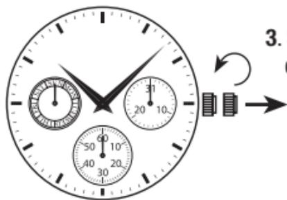
**3. Set the date by rotating the crown in counter-clockwise direction (Quick change function).**
